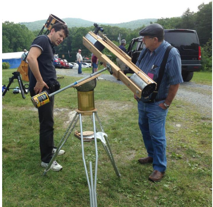
One more look at the Fullum Dob (above), if only to admire the craftsmanship of the eyepiece rack and its shadow. A very odd Newtonian, all crutches and cans and a cooking bowl for the mount, and yet perfectly balanced to attract inquiring minds (right).
