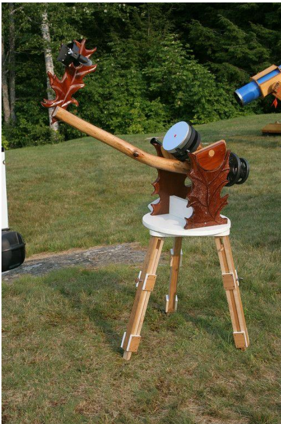
A wide-open, single-truss, stripped-tree-branch and leaf-motif design. Even the collimation could feel a breeze.
