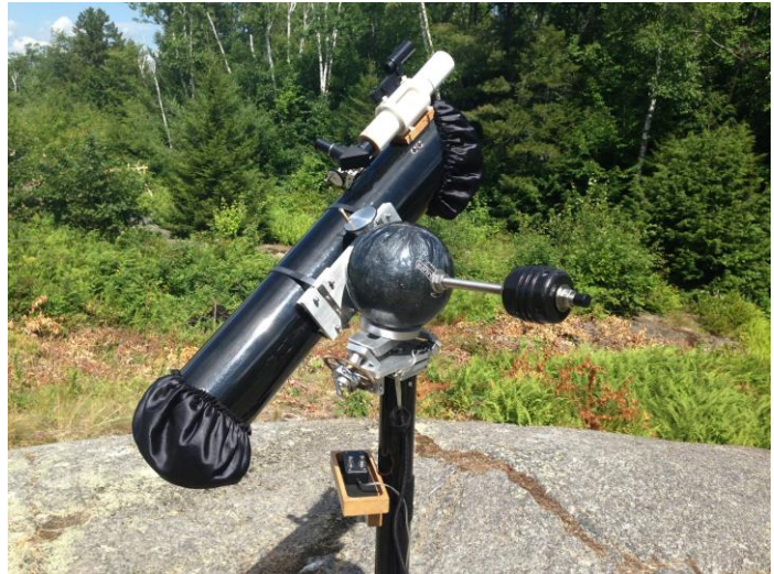
Not a bino-viewer, but a bino-scope (left), made out of a pair of (possibly) 8" Coultter OTAs. Apparently the view was great! Meanwhile, a bowling ball had been put to good use, with a Poncet tracking platform (right). Only one toe-saver was supplied.
