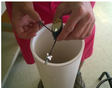
Greg Luber, Tomas Larsen and Gabe Rodriguez-Polanco went from figuring how to extend the (shorter) spider vanes of the Tasco's secondary mirror assembly to fit the new (and unpainted) PVC tube on Day 1, to doing a laser collimation check on their new Dobsonian Reflector on Day 3.
