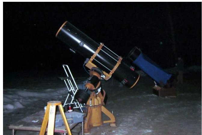
The trademark 12.5" Newtonian on its EQ mount, and the blue-shrouded 17.5" Newtonian (in the back) on a Dobsonian mount. (All photos: Bonnie Derek)
